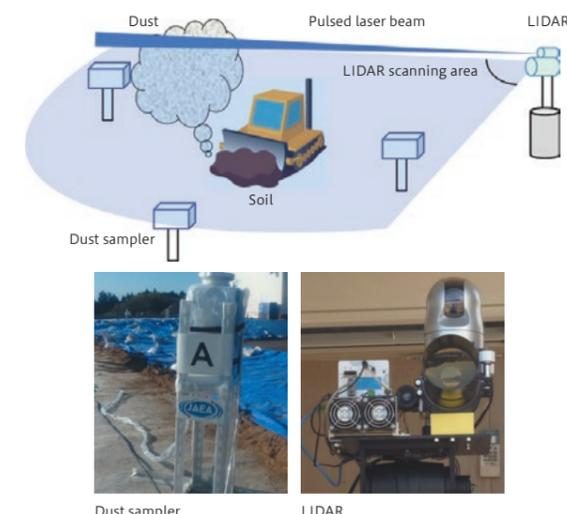
"LIDAR" is a technology to measure the distribution of dust using harmless lasers.
