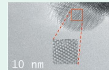
TEM image of hillock in  $\text{BaF}_2$  formed by heavy ion irradiation
