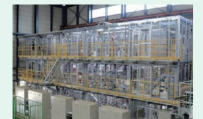
Continuous hydrogen production test facility made of industrial materials
