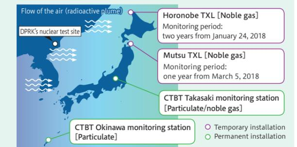
Installation maps of CTBT radionuclide monitoring stations and mobile noble gas measurement systems operated by JAEA
