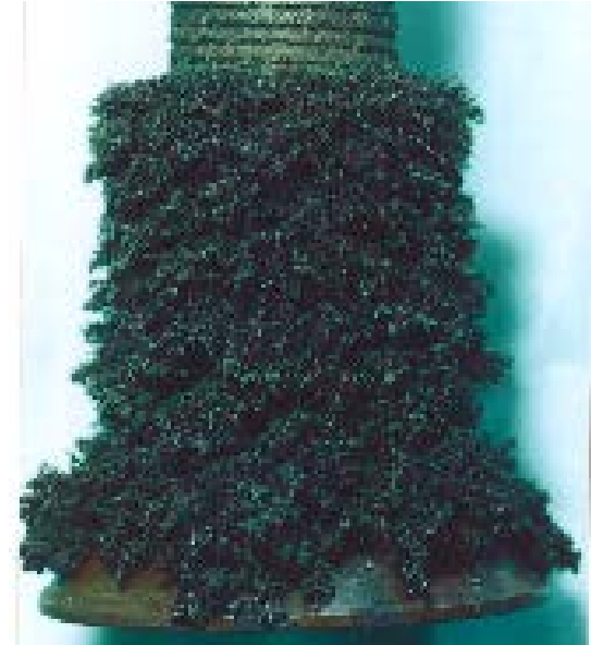
1 kg metal uranium deposited by electro-refining (in cooperation with CRIEPI)
