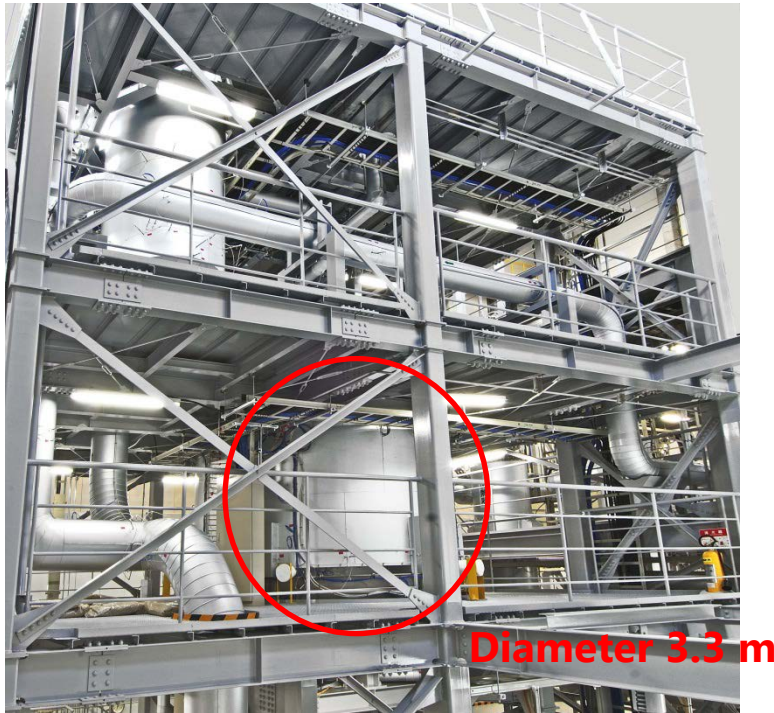
Sodium test of the full-scale EM pump for Toshiba Small FR, 4S
