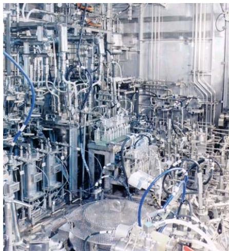
Experimental apparatus in NUCEF for tests of DIDPA extraction process with real HLLW from LWR SF
