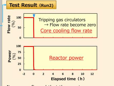
It was confirmed that the reactor power decreased to about zero automatically and reached to stable state without activating the reactor shutdown
