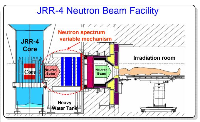
The energy spectrum of a neutron beam is designated to any of thermal or epithermal group by the neutron spectrum variable mechanism according to the need in each trial.
