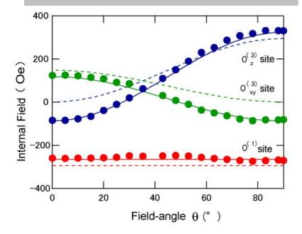
Field-angle dependence of the internal field at O sites in  $NpO_2$ . The solid and dotted lines are the results of model calculations with and without the contribution from the field-induced magnetic octupolar ordering, respectively. Yo Tokunaga Advanced Science Research Center, Japan Atomic Energy Agency
