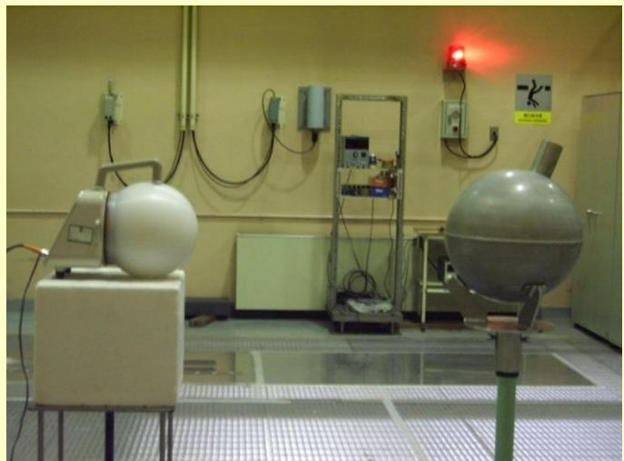
**D<sub>2</sub>O moderator (For D<sub>2</sub>O-Cf neutron field)**
