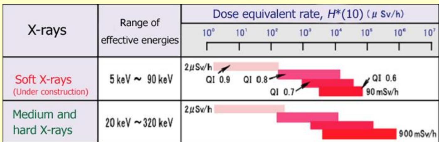
QI: Quality Index = Effective energy of X-rays / Maximum energy of X-rays generated
