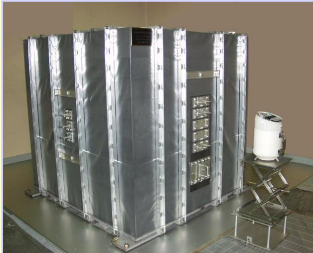
**Graphite pile (for thermal neutrons)**
