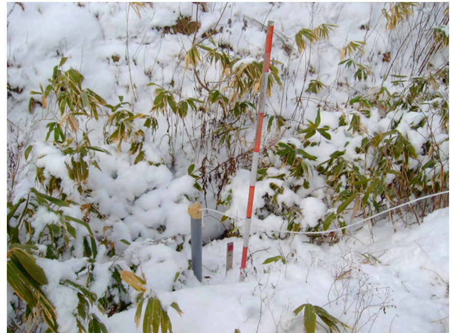
Gas collection using vinyl chloride pipe
