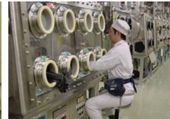
Data acquisition using atmospheric controlled chamber under reduced condition
