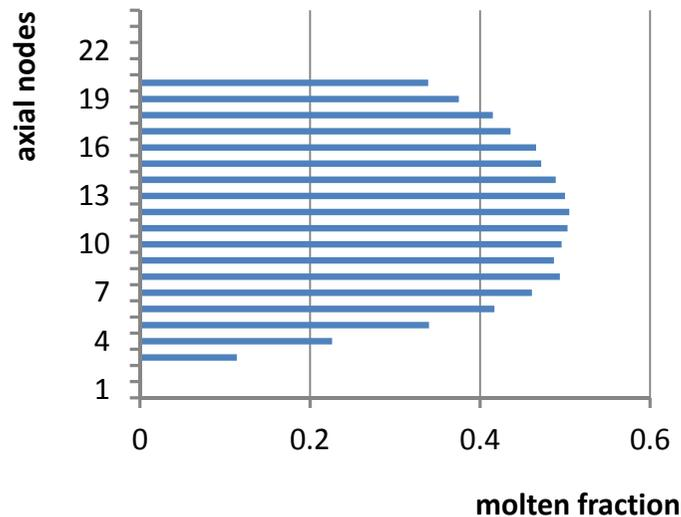
Molten fraction in drive channel in UTOP (assumed quick and large reactivity insertion)
