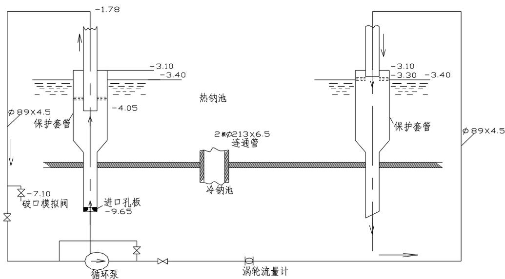
Illustrative diagram of anti-siphon device and the primary auxiliary pipe
