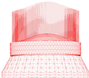
Integrated FEM model of core, GP and CSS
