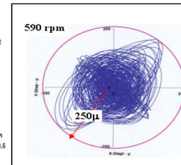
HSB orbit under SSE to ensure no impact
