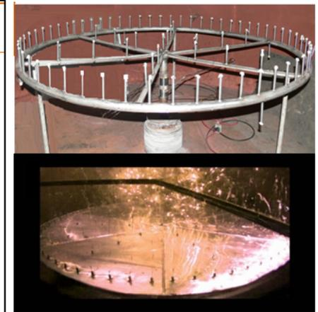
SOCA Facility to simulate Na fire scenario on top shield
