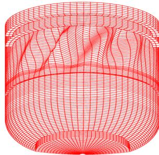
Buckled mode shapes of RA vessels under seismic loadings
