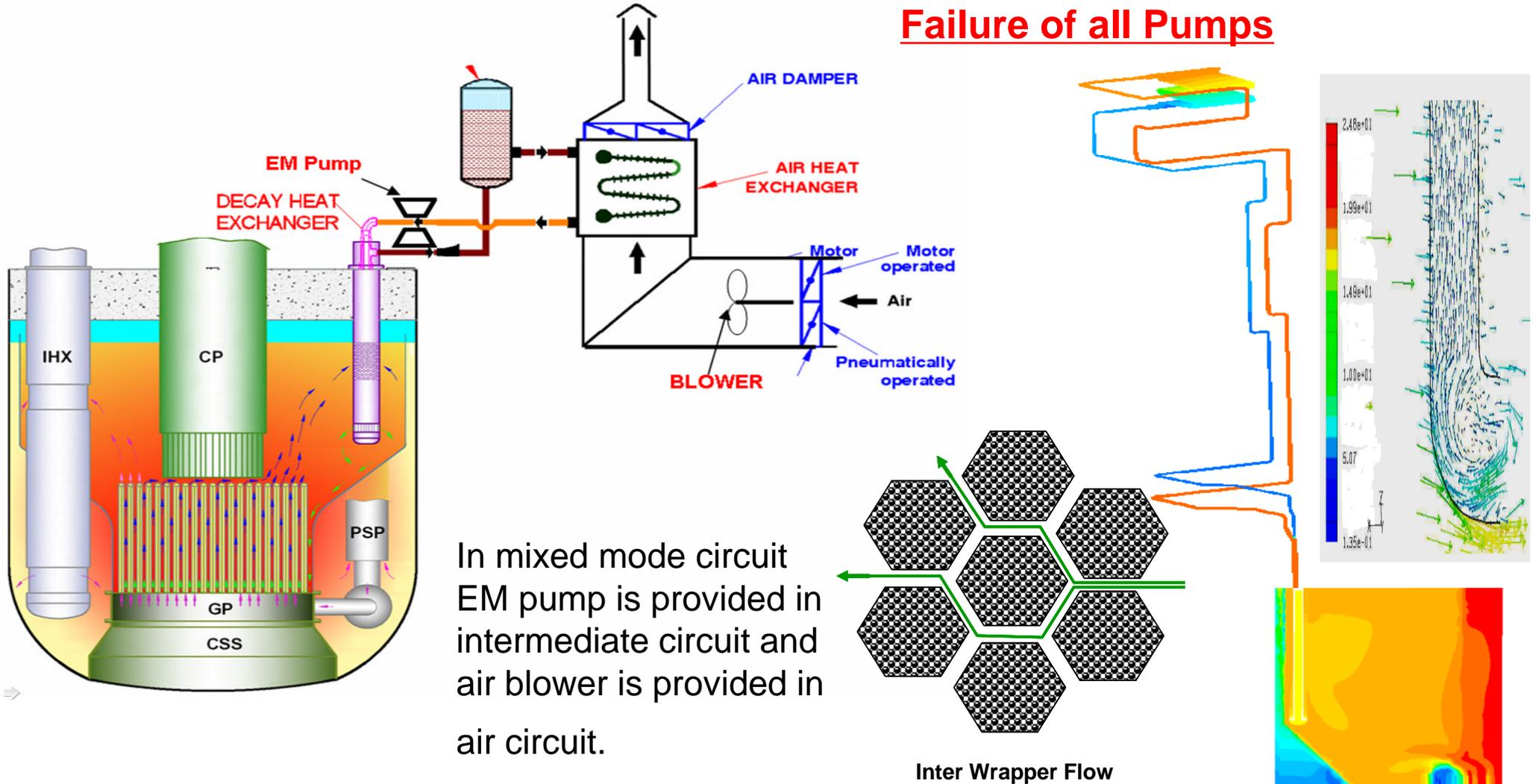
*Analysis with multi-dimensional model for pools with inter-wrapper space (StarCD) and 1-D model for equipments and piping (DHDYN).*
