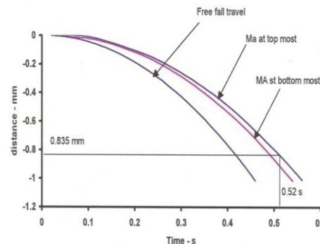
Drop time of absorber rods during SSE
