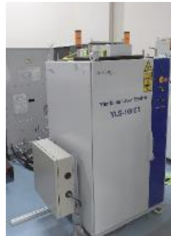
10kW CW laser oscillator
