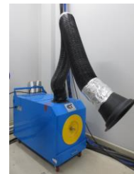
Local exhaust device
