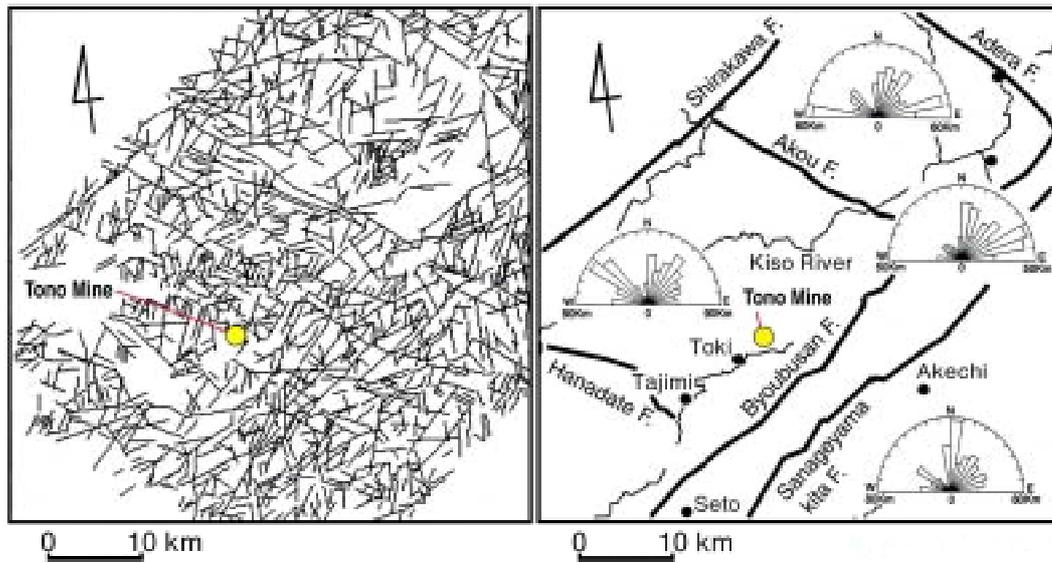
**Figure 4.1(1) Lineament interpretation in the Tono district and lineament rose diagram for each fault-bounded block (top)**
