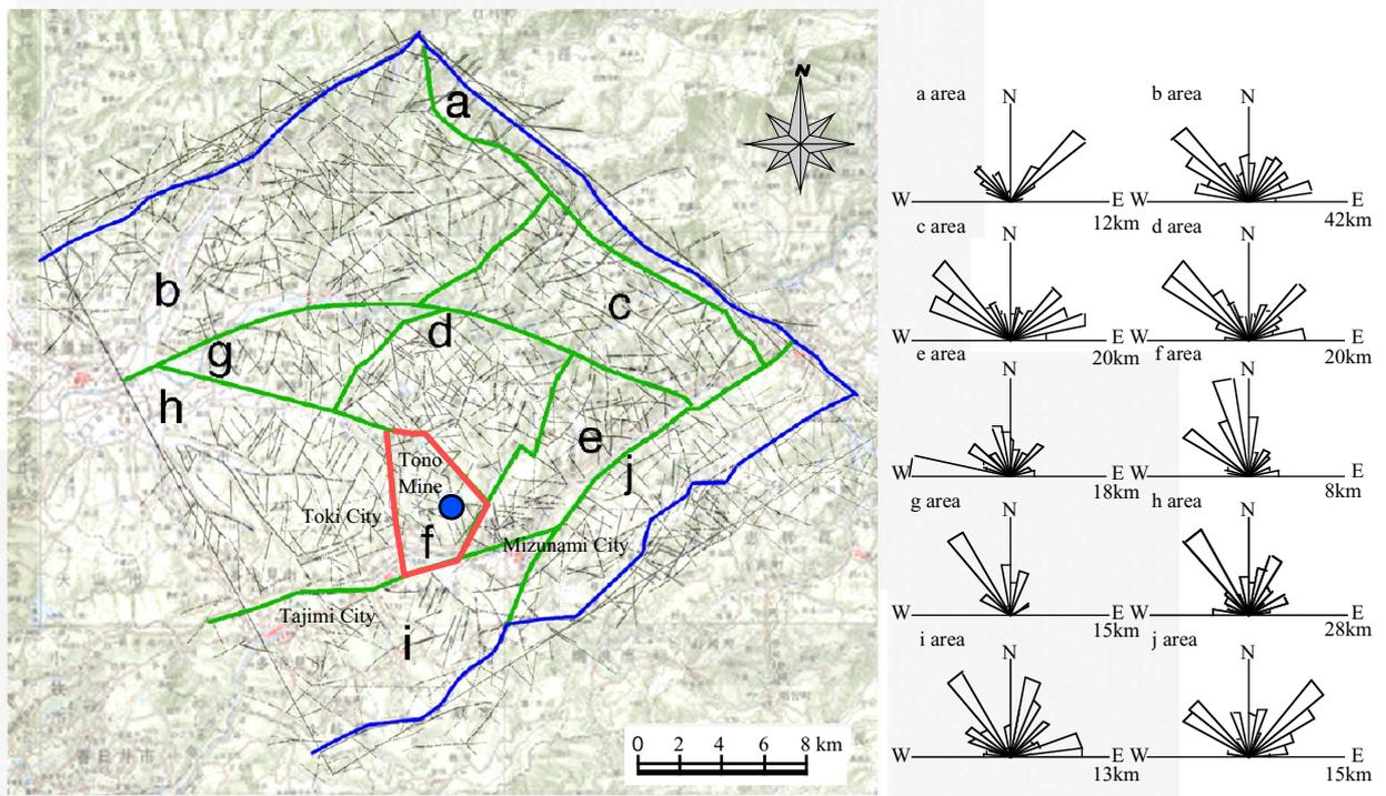
**Figure 4.1(2) Division based on the result of the lineament interpretation and rose diagram**
