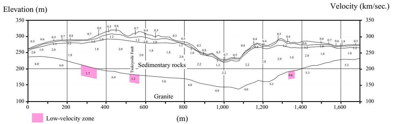
Figure 4.5 Distribution of seismic wave velocity (Line-R-1)<sup>15)</sup>
