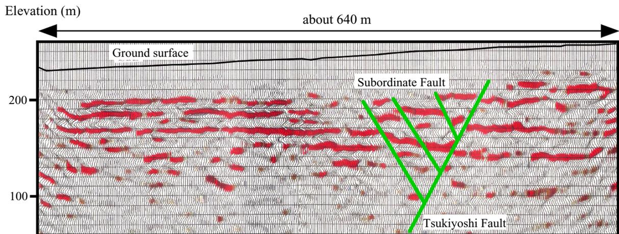
Figure 4.6 Cross section of survey line A-B (Line-1)<sup>15)</sup>
