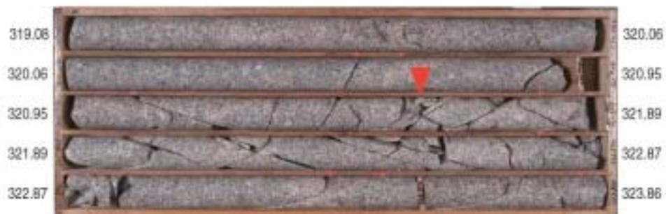
(a) Section of drillcore from a water inflow point (depth range 319.08 to 323.86 mbgl)
