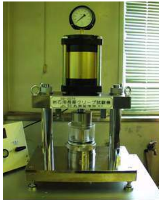
Fig. 4.7.4-5 Test equipment for uniaxial creep test
