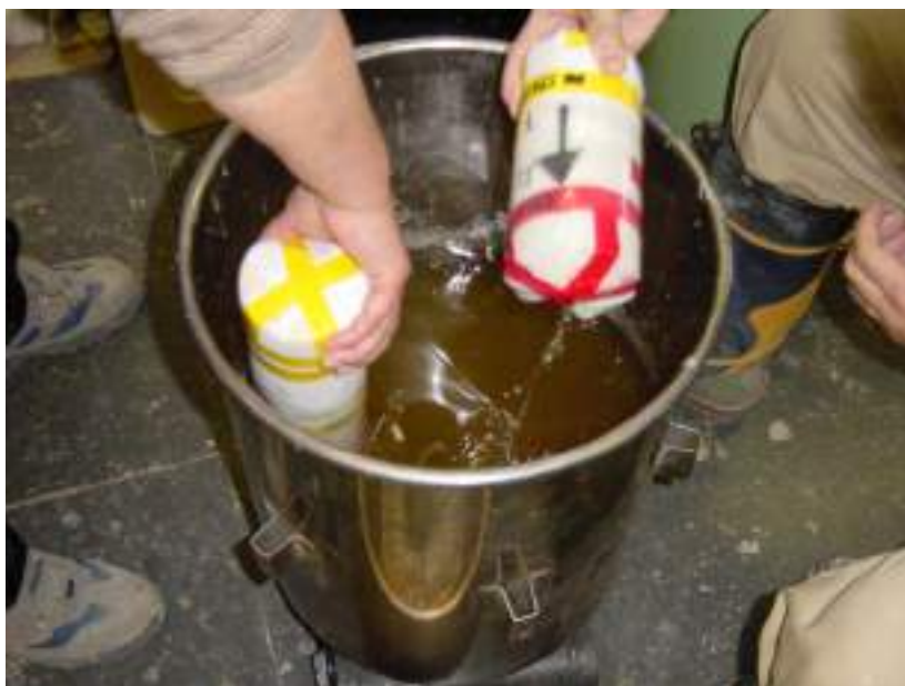
Fig. 4.3.2-1 Pretreatment of rock sample for porewater squeezing
