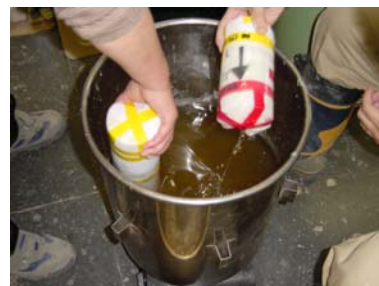
Core sealing with plastic film, Al-foil, cotton cloth and wax (Ota et al., 2007)
