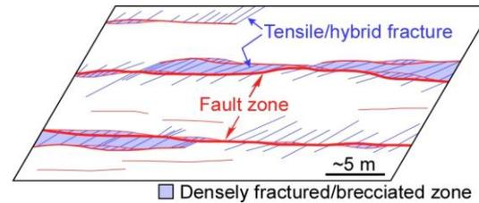
Fault connectivity based on outcrop & borehole data
