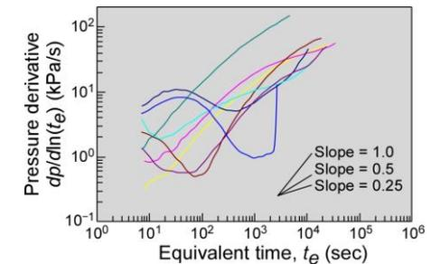
Pressure derivatives from packer tests for faults
