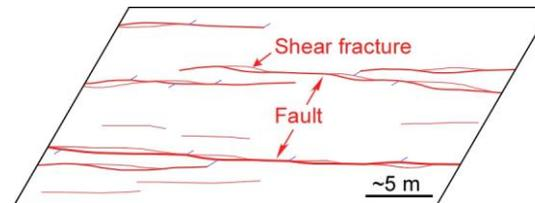
Fault connectivity inferred from borehole data
