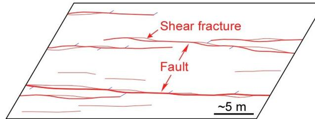
Schematic image depicting poorly connected faults (from borehole data)
