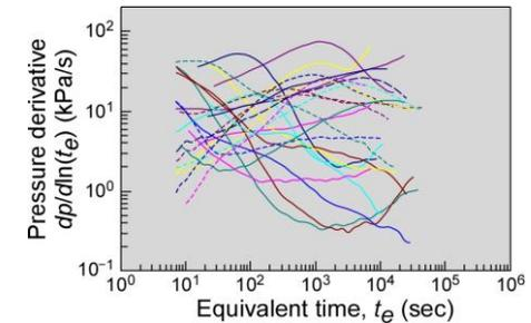
Pressure derivatives from packer tests for faults
