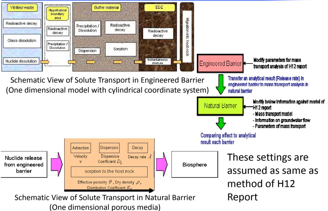
Schematic View of Solute Transport in Natural Barrier
