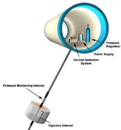
Layout of the long term diffusion test at GTS
