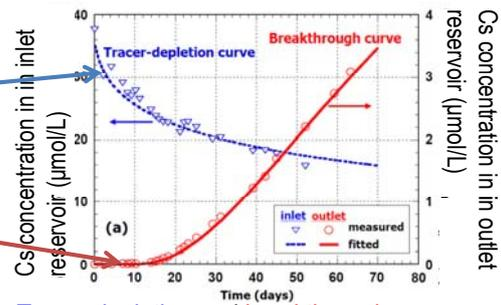
Tracer-depletion and breakthrough curve
