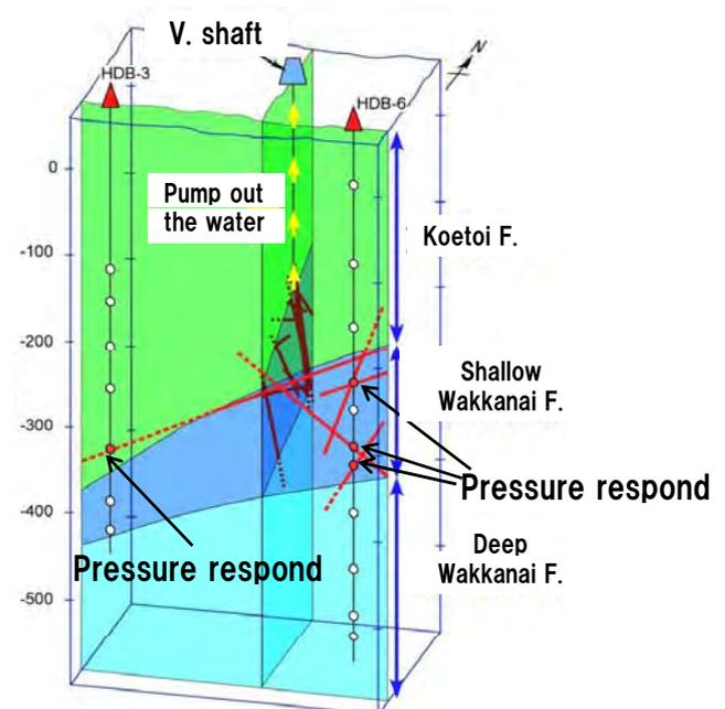
Location of pressure response zones correspond to inferred hydrogeological structure by hydrogeological model. Furthermore large scale hydraulic disturbance will be occurred after shaft sinking below 250m level.
