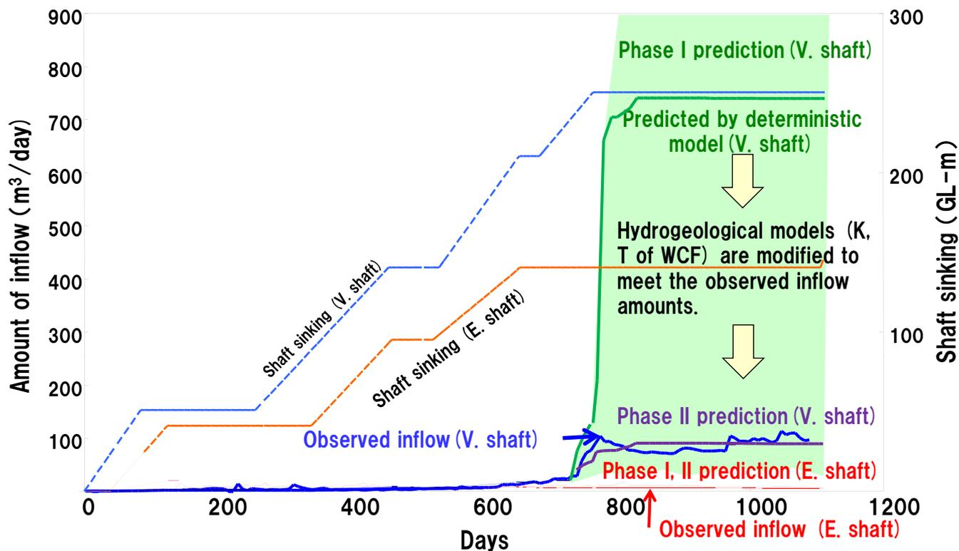
Modified model is used to predict the inflow amount at deeper than 250m.
