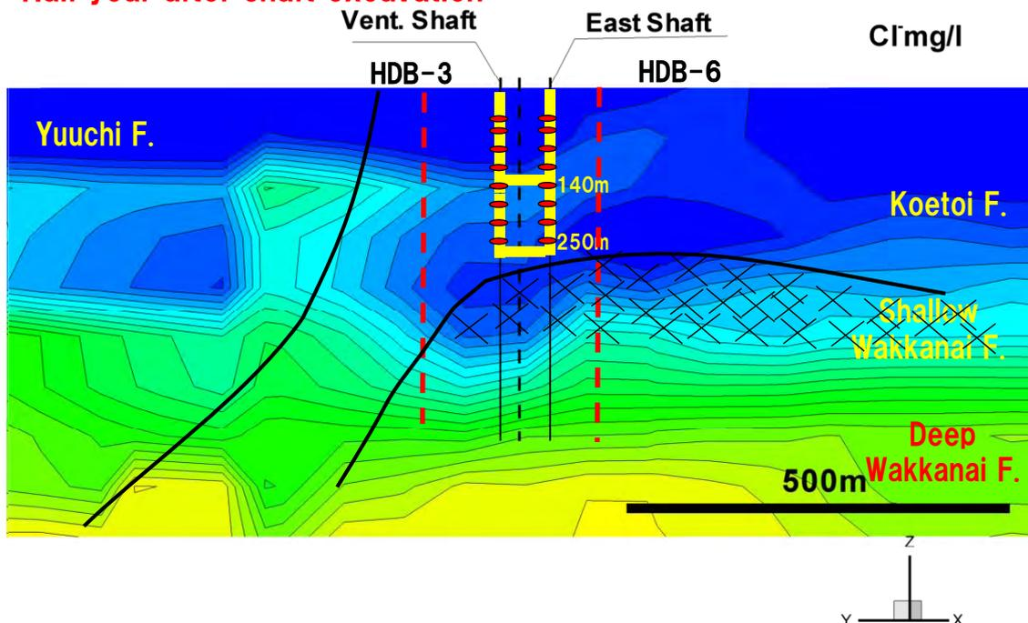
Chemical composition around the depth of 250m is changing by groundwater inflow into shafts. Such observation is used to develop the methods of hydro-chemical coupled modelling.
