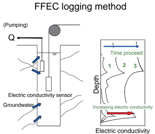
1. Replace borehole water by de-ionized water
