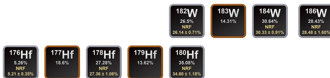
Fig. 4 Isotopic analysis obtained by the NRF method for natural Hf and W metals.
