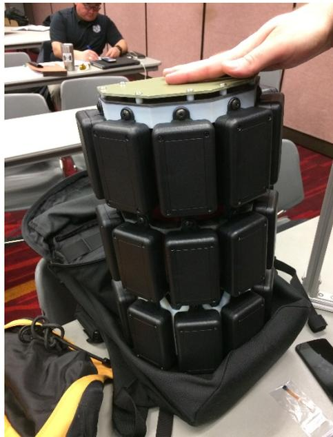
Open system architecture and ergonomically designed backpack and vest device that enables identification and localization while seamlessly integrating operationally deployed detection networks.
