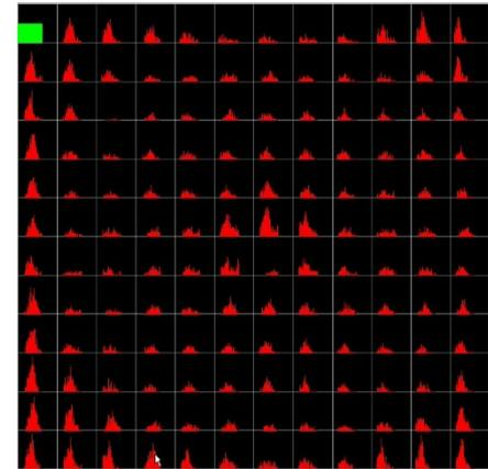
Transmission image (50 yen coin) measurement using <sup>241</sup>Am source (60 keV) and energy spectrum
