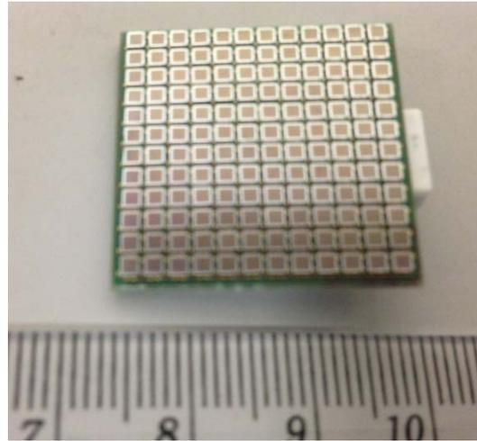
SiPM 1.6 x 1.6 mm<sup>2</sup> of 1.9 mm pitch based on PM1150 (KETEK)
