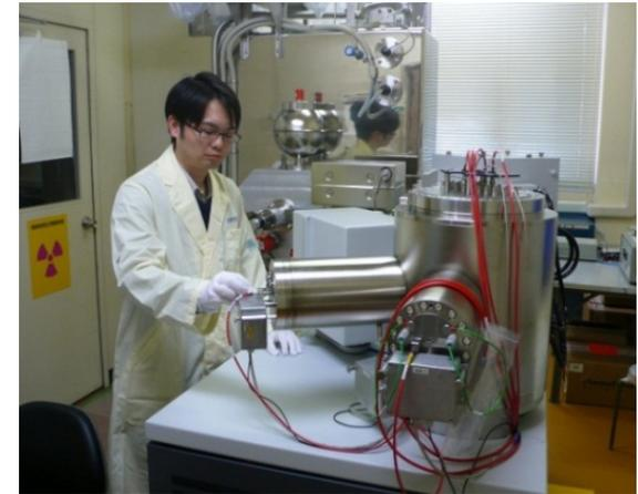
Thermal Ionization Mass Spectrometry
