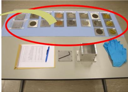
Au, W, Rh, Cu, Co, Mn samples (plates) with different thicknesses were prepared.
