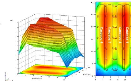
Neutron survey data in a cascade hall (before holdup recovery)
