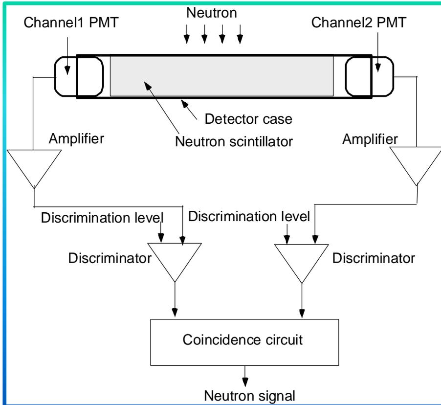
Neutron Detection using  $\text{ZnS}/^{10}\text{B}_2\text{O}_3$  Ceramic Scintillator
