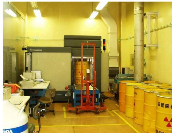
Measurement system of waste drum
