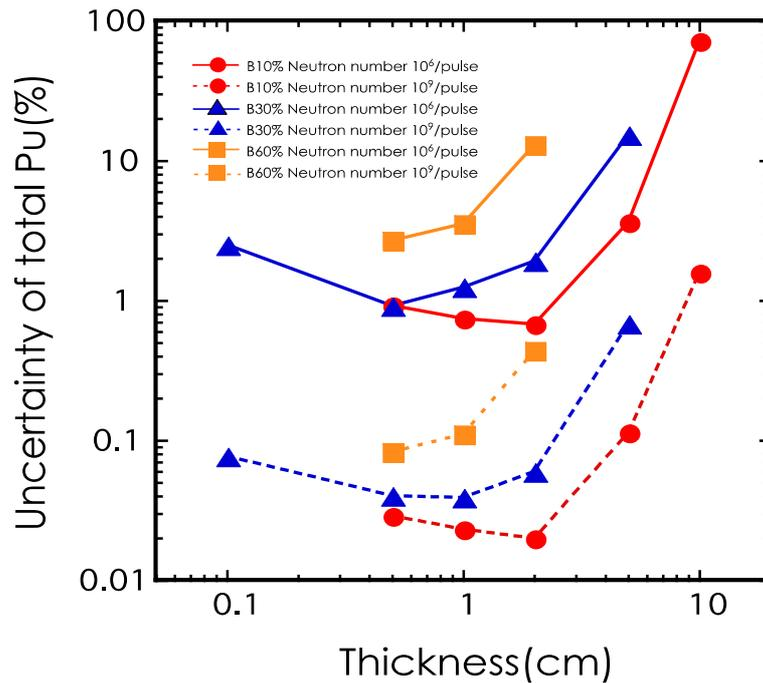
Figure 7. Counting statistics uncertainty on the total Pu amount in the sample as a function of the sample thickness for different boron concentrations.
