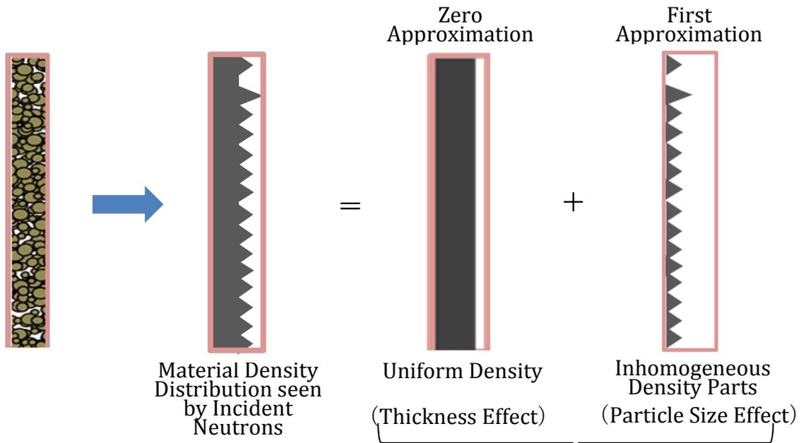
**Impact of systematic effects on the accuracy of NRD is about 2% for samples with a thickness  $\leq 2$  cm. The accuracy can be reduced by improving the required nuclear data, i.e. resonance parameters.**
