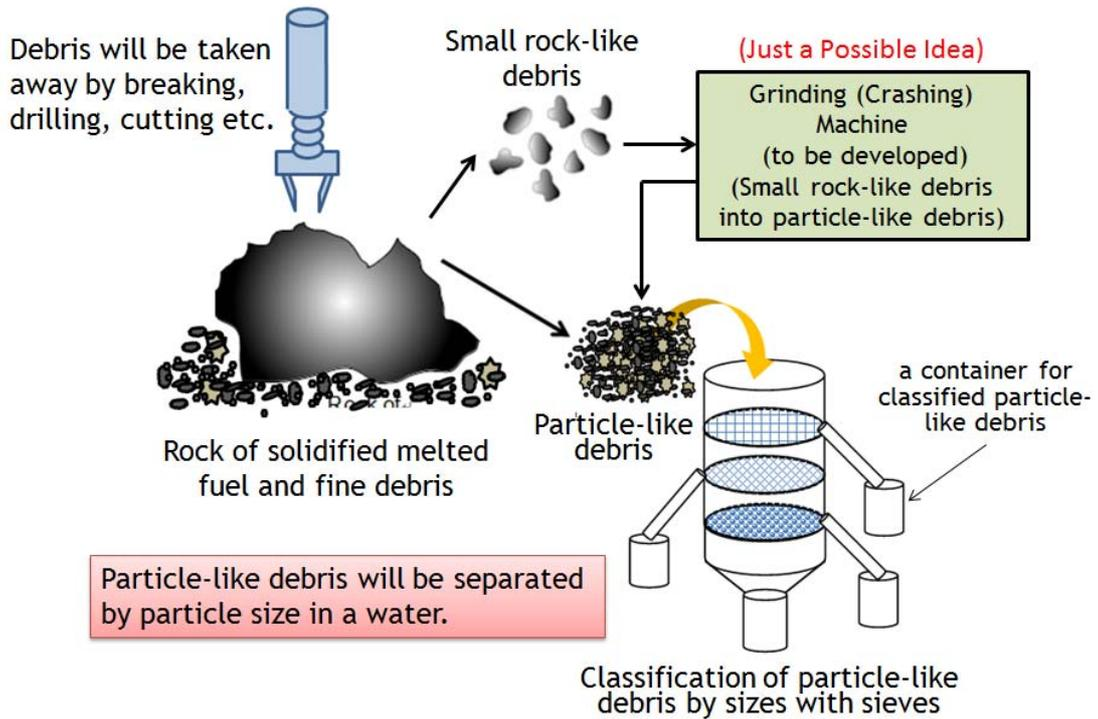
Figure 10 (a) Collection of particle like melted fuel debris
