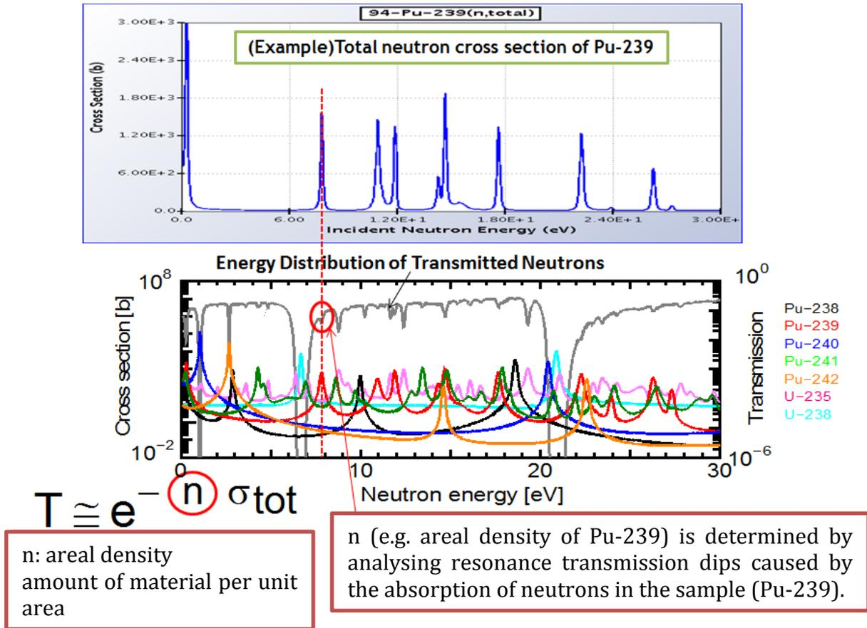
Figure 2 Determination of the areal density (e.g. Pu-239) by NRTA.
