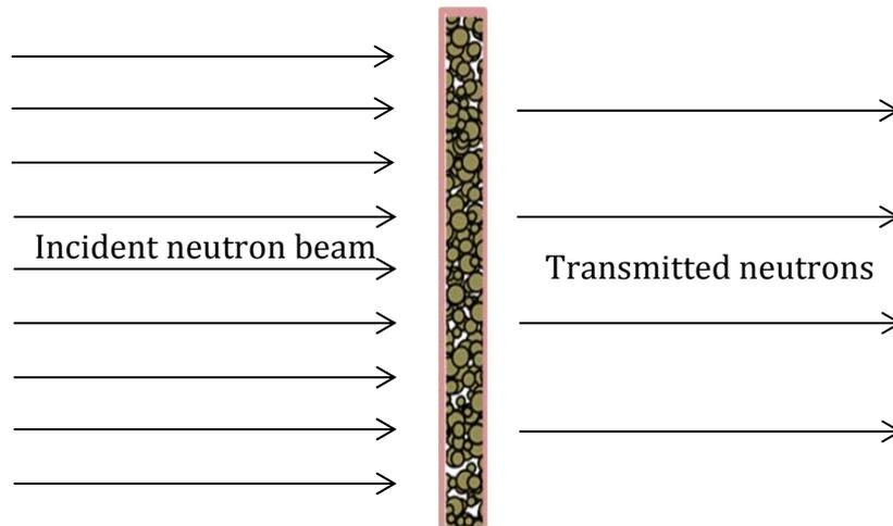
A thin disk container with particle like melted fuel debris
