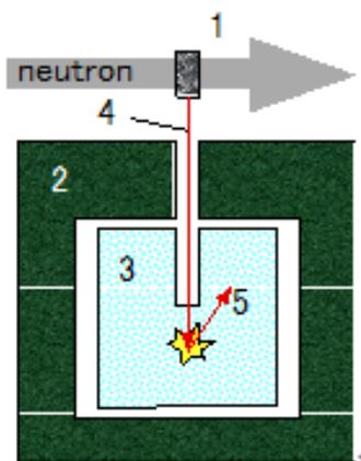
(a) An well-type gamma-ray spectrometer: (1) a sample, (2) a passive shield, (3) a well-type  $\text{LaBr}_3$  detector, (4) a gamma-ray, and (5) a scattered gamma-ray.
