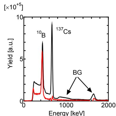
(b) Identification of  $^{10}\text{B}$  by the detection of prompt gamma-rays using a (5" x 5")  $\text{LaBr}_3$  detector at GELINA.
