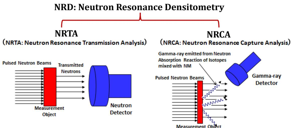
NRTA: Quantification of (U/Pu) isotopes by analysing neutron transmission resonance dips. The results of NRCA are used to account for the influence of neutron absorbers on transmission profiles obtained with NRTA.
