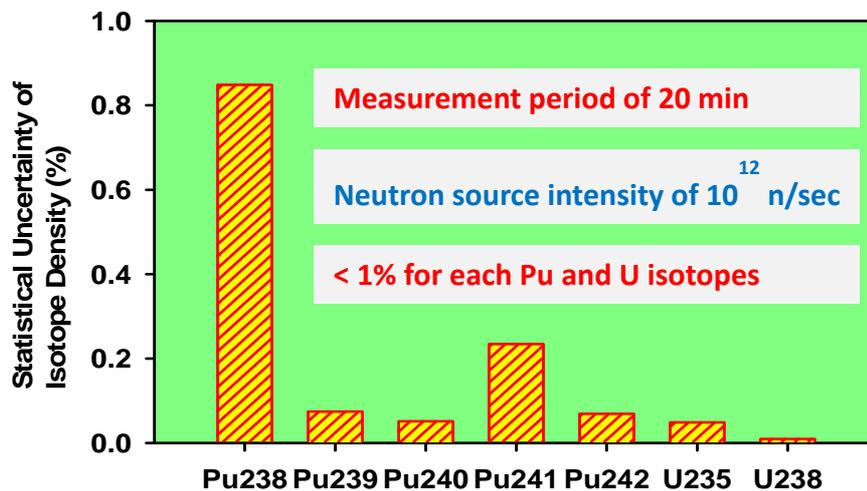
Figure 5 Achievable counting statistics uncertainty for NRTA on melted fuel debris containing B-10 as matrix material.
