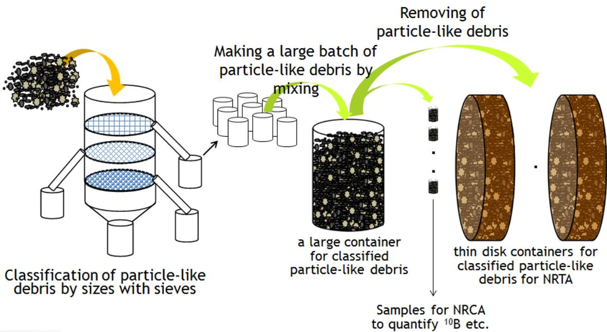
Figure 10 (b) Preparation of measurement objects for NRD
