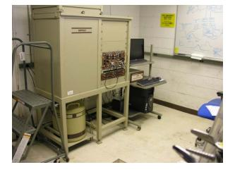
Compton Suppressed Gamma-ray Spectrometry
