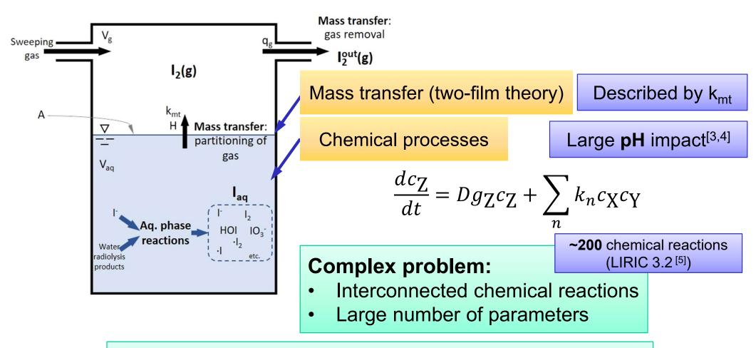
How significant are the separate contributions of chemical and mass transfer processes?
