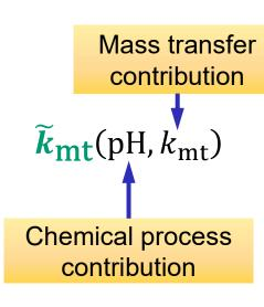
$$\frac{d}{dt}f_{I_{2}(g)} = A\tilde{k}_{mt} \left[ \frac{f_{I(aq)}}{V_{aq}} - \frac{H}{V_{g}} f_{I_{2}(g)} \right] - q_{g} \frac{f_{I_{2}(g)}}{V_{g}}$$
