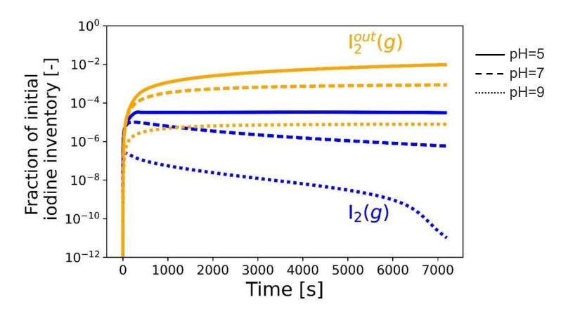
The amount of gaseous iodine that escapes from the aqueous phase decreases with increasing pH
