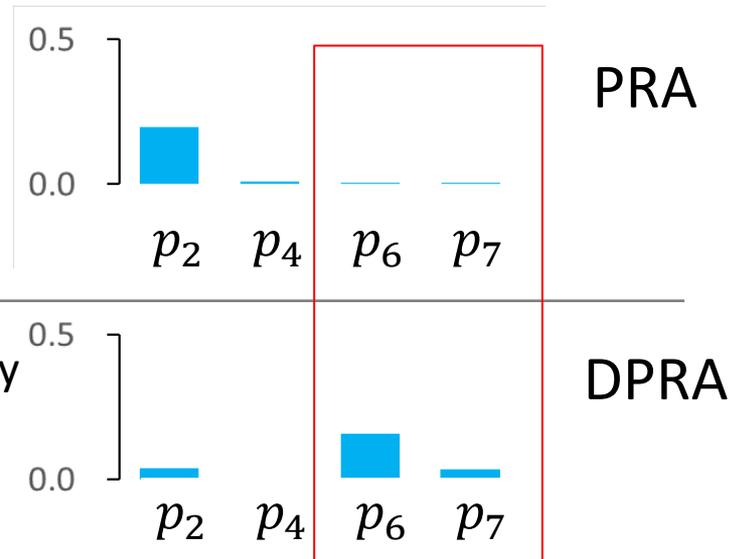
SRV tends to fail with fewer open/close cycles ( $p_{srv|SBO} > p_{srv}$ ), resulting in the change of CCDP distributions
