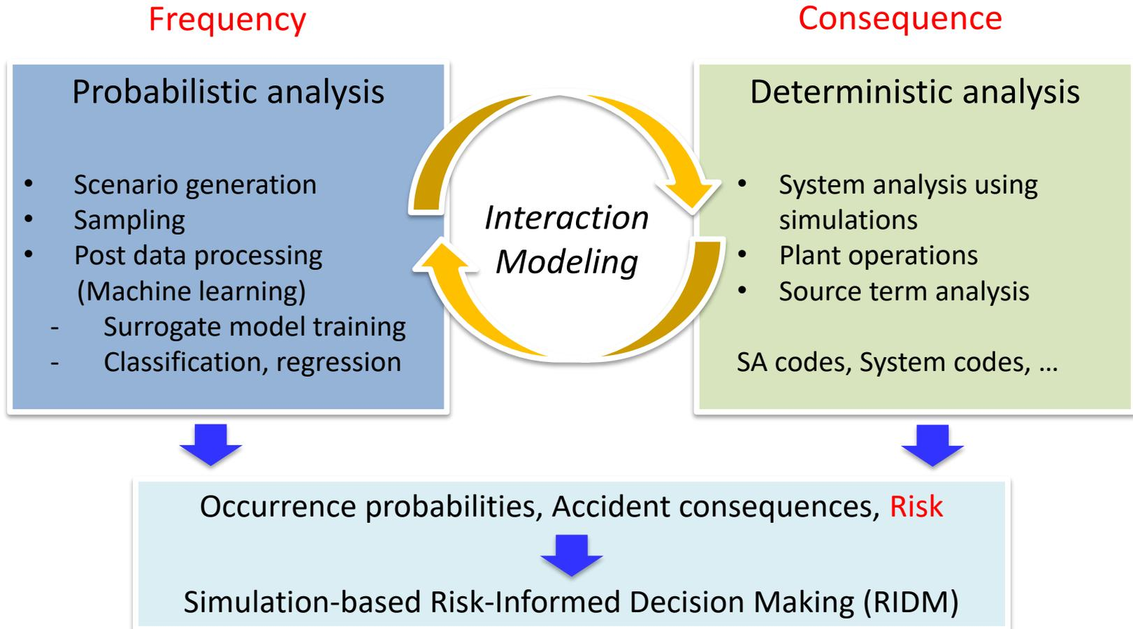
The method refers to the RISMIC (LWRS, USDOE) approach developed at INL, but with a unique accident scenario generation mechanism considering frequent simulation interactions
