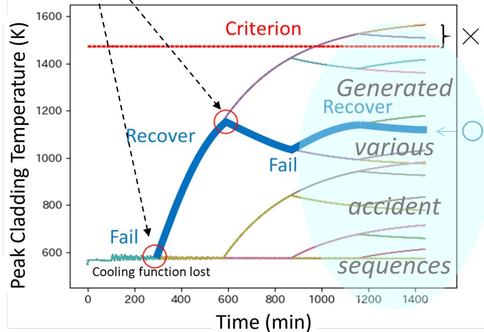
Problem: failure probabilities are simplified as independent from accident progression ► **JAEA Solution**: scenario-dependent failure modeling (**Interaction**)
