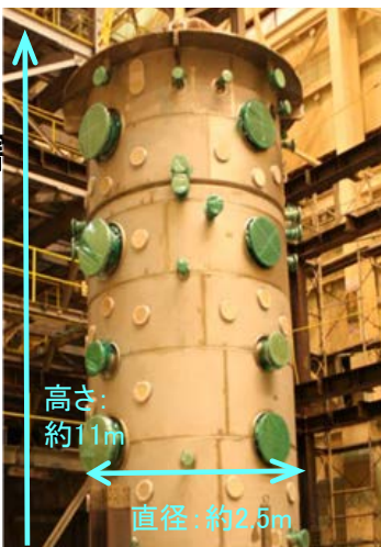
CIGMA (Containment InteGral Measurement Apparatus) の外観
