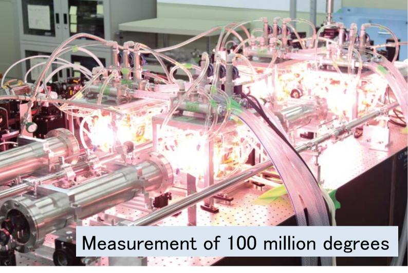
(Above) In order to produce nuclear fusion energy, which is called "Sun on Earth", plasma of ultra-high temperature exceeding 100 million degrees is required. A special laser thermometer as depicted above must be used to measure the temperature as high as 100 million degrees.
