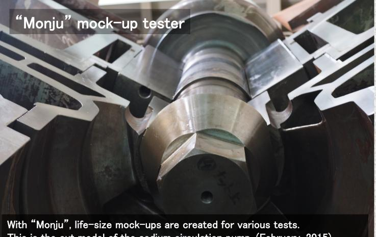
This is the cut model of the sodium circulation pump. (February, 2015)
