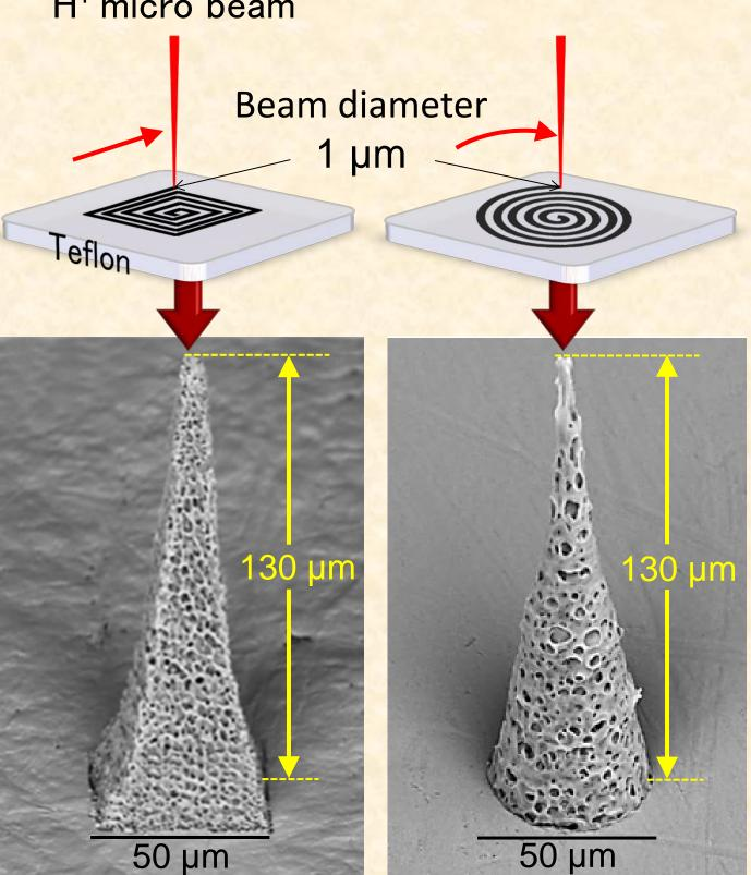
Extremely thin rays of particles moving at 30,000 km/sec are irradiated to the Teflon plate from the center to the peripheral in spiral. Then, the irradiated parts rise forming a shape like soft-serve ice cream, which become a cone or pyramid as depicted above http://jolisfukyu.tokai-sc.jaea.go.jp/fukyu/mirai-en/2013/img/honbun/13-19.jpg
