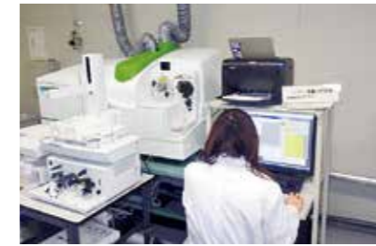
ICP-Mass Spectrometer This provides high-sensitivity multi-element analysis using plasma as an ion source. It enables information on trace element concentration in environmental water to be obtained.
