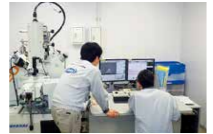
Element Analyzer This irradiates a sample surface with an electron beam to observe the surface structure and perform element analysis. It is used, for example, to obtain information on the chemical composition of radioactive substances absorbed by soil.
