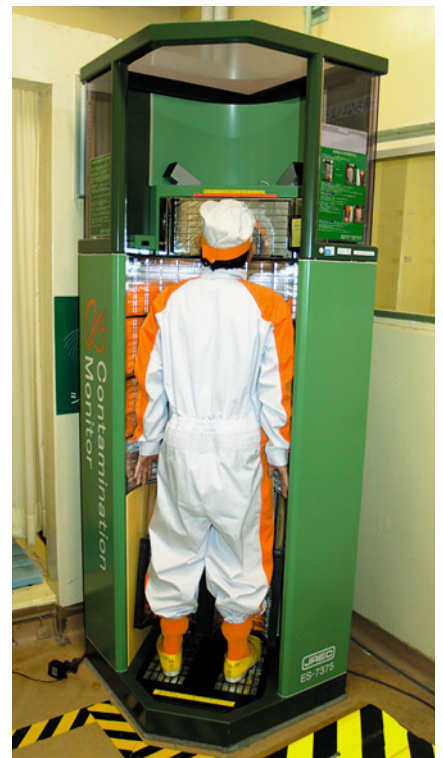
▲ \alpha/\beta Contamination monitor (Monitoring of the surface contamination)
