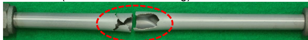
Split after quenching due to oxidation & embrittlement
