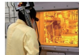
Handling of an experimental apparatus installed in a concrete cell
