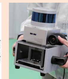
iRIS for visualization of radioactive contamination at decommissioning sites through 3D mapping
