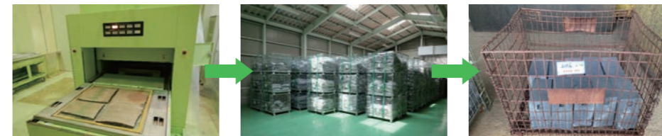
Radioactivity measurement for clearance | Storage of materials after measurement | Processed metal materials (ingots)
