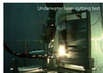
Development of remote laser cutting technology at Fugen
