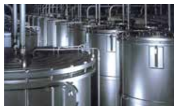
Gas centrifuge at uranium enrichment demonstration plant DOP-2, opened in 1989
