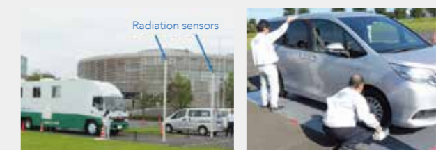
Radioactive contamination screening test for automobiles using gate-type radiation monitors and ordinary radiation survey meters
