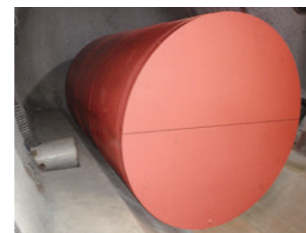
[Horonobe] In-situ demonstration of PEM (Prefabricated Engineered barrier system Module)
