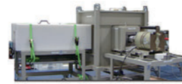
Delayed gamma-ray analysis test equipment capable of measurement of nuclear materials contained in highly radioactive and complex materials
