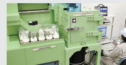
Germanium (Ge) semiconductor detector for low-energy gamma rays equipped in the workshop.
