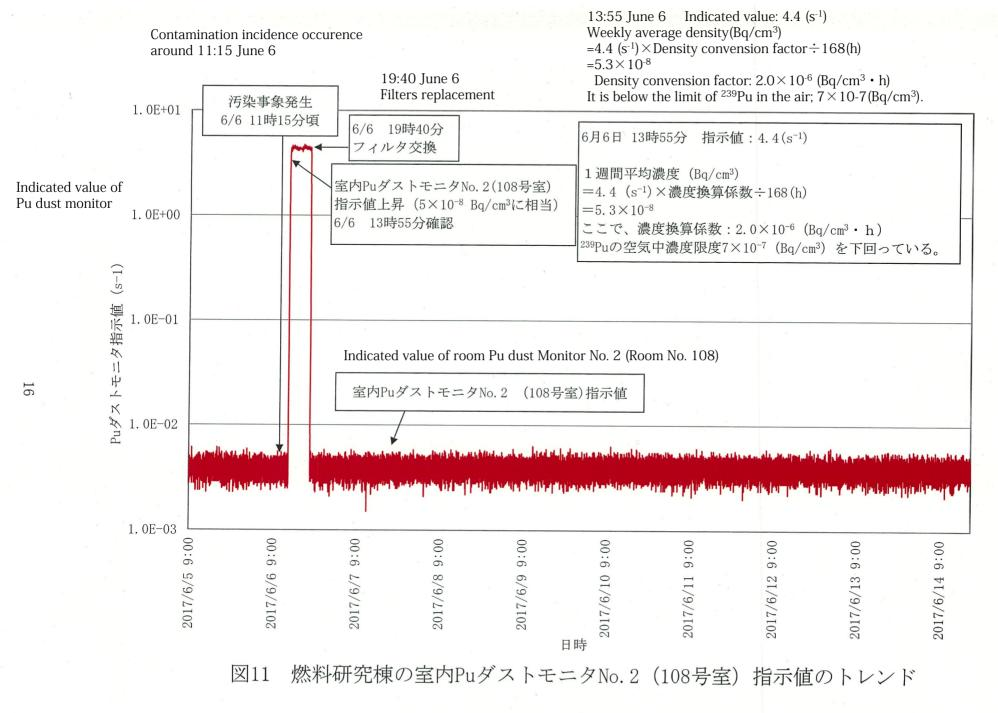
Fig.11 Indicated value trend of room Pu dust monitor No.2 (Room No. 108) at PFRF
