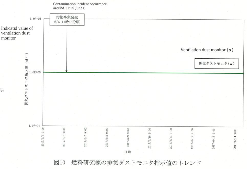
Fig.10 Indicated value trend of ventilation dust monitor at PFRF
