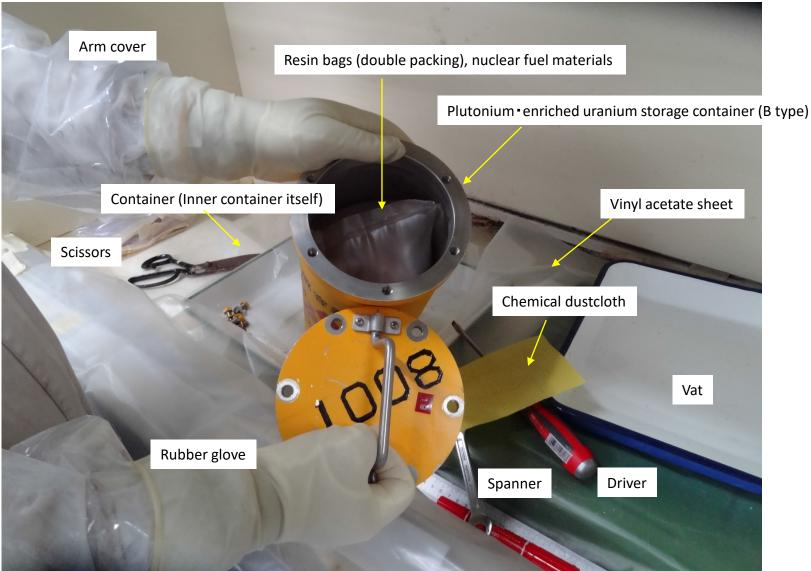
The vat and scissors were not used for this work. Instead of using a bat, the inner floor of the hood is cured with the vinyl acetate sheet.
