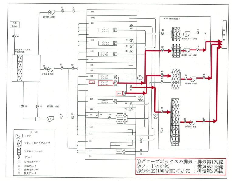
図15 燃料研究棟の排気系統図 Fig. 15 Ventilation system at PFRF ①1st system: Ventilation of glove boxes
