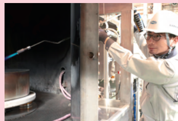
Apparatus for Evaluating Clogging Effect of HEPA Filter on Confinement Capability Under Fire Accident (ACUA)
