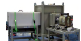
Delayed gamma-ray analysis instrument, tested at the JRC Ispra (Italy)
