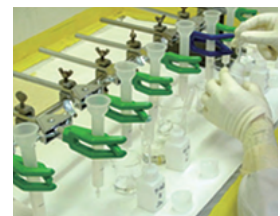
Analysis of ^{90}\text{Sr} using strontium adsorption resin
