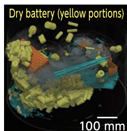
Identification of a dry battery (mercury) based on the characteristics of three-dimensional geometries
