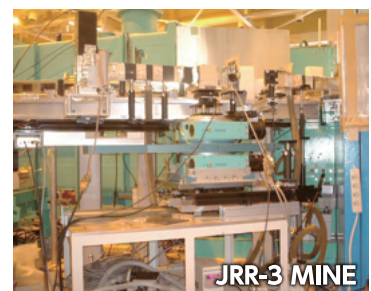
JRR-3 MINE Neutron reflectometer at JRR-3*
