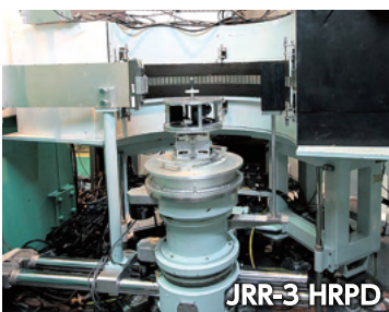
JRR-3-HRPD Neutron diffraction equipment at JRR-3*
