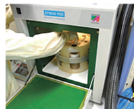
Sample dissolution based on a microwave digestion
