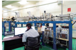
[Tono] A dating equipment at TGR (Pelletron Accelerator mass spectrometer, JAEA-AMS-TONO-5M)
