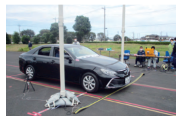
Measurement experiment using radiation portal monitor for vehicles
