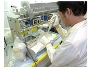
Analysis of ^3\text{H} and ^{14}\text{C} based on a combustion method
