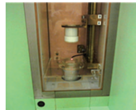
Measurement of gamma rays based on a high-purity Ge detector
