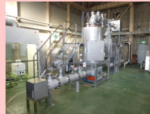
Apparatus for Evaluating Clogging Effect of HEPA Filter on Confinement Capability Under Fire Accident (ACUA)
