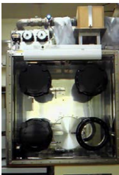
Fig: Sample Loading Box
