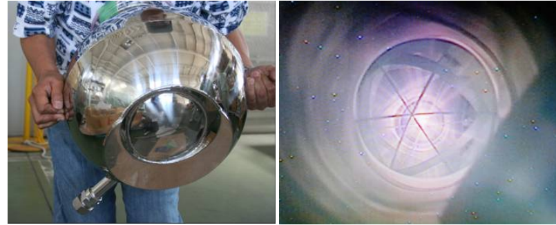
Compact DD-IEC neutron source and discharge photo inside
