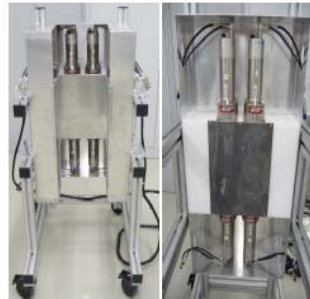
System based on a EJ309 scintillator
