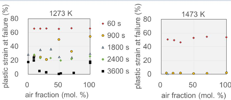
Significant reduction of the plastic strain at failure due to large H pick-up
