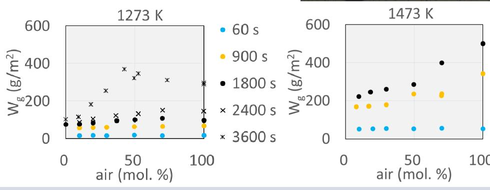
Effect of the air fraction on W<sub>a</sub> is substantial: tendencies differ depending on T (effect of partial pressure of O<sub>2</sub> & flow rate)
