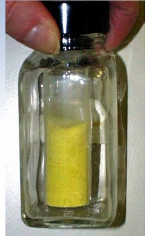
High purity uranium oxide product recovered from used nuclear fuel using the UREX+ process
